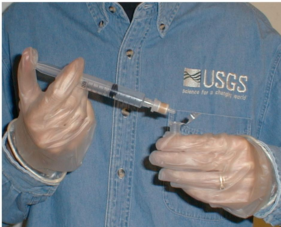
Figure 2. Hexavalent chromium field separation.
