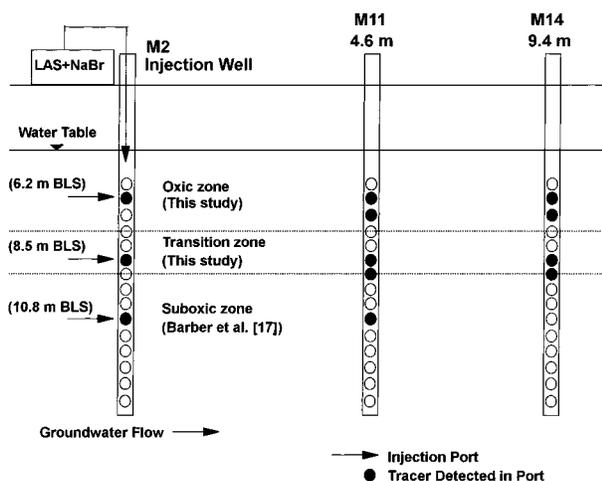
FIGURE 1. Multilevel sampling wells used during the oxidic, transition, and suboxic tracer tests including the locations of the injection well (M2), the downgradient monitoring wells M11 and M14, and sampling ports.
