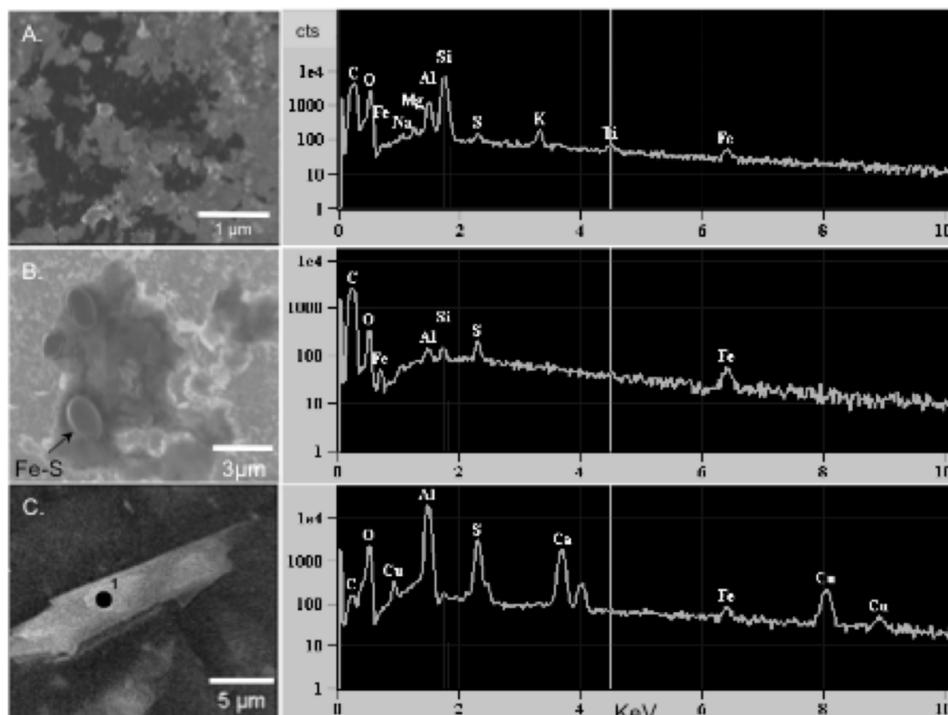
**Figure 2.** SEM images using 30 kV, 2.1 nA current, (A) Clay particles on graphite (dark substrate). EDS (right) shows elements over a rastered area, (B) Close up of Fe–S spherules in aluminosilicate matrix. EDS spectrum is rastered over spherules, (C) Lath shaped particle with high Ca, S, and O (black dot) interpreted as gypsum or jarosite.
