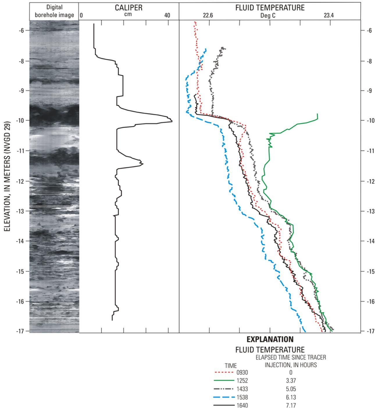
**Figure 8.** Open and oriented view of borehole wall image from digital optical borehole image (OBI) log, caliper log, and fluid temperature versus depth for discrete times in observation well G-3772.
