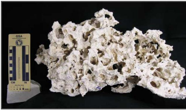
**Figure 3.** Photograph showing touching-vug porosity in a Miami limestone rock sample.
