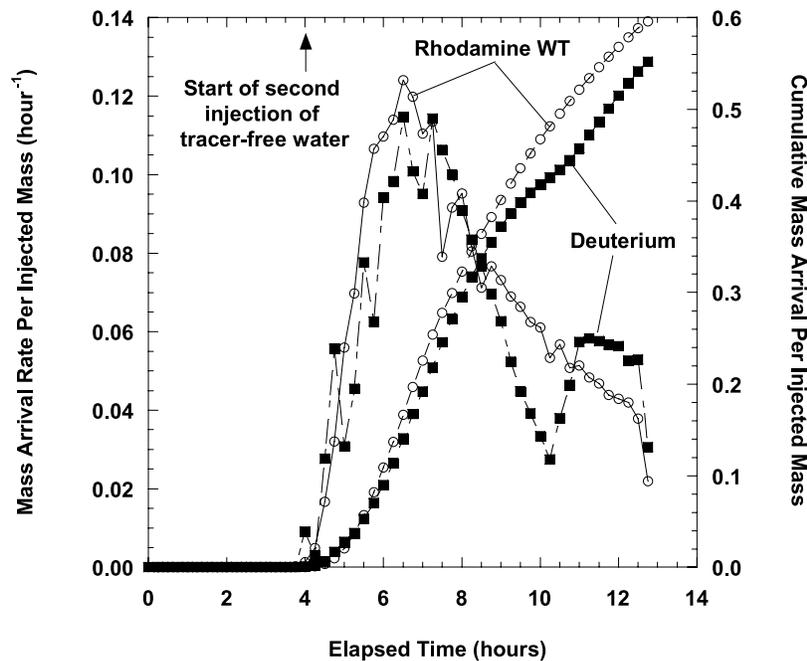
**Figure 7.** Normalized rate of mass arrival per injected mass and cumulative mass arrival per injected mass for RWT and  $^2\text{H}$  at production well S-3164 versus elapsed time from the start of the tracer injection.
