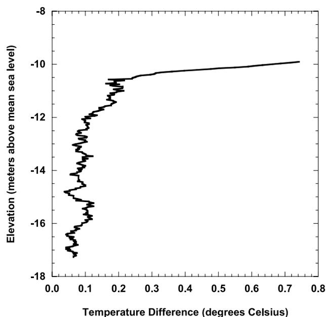
**Figure 9.** Recorded difference in fluid temperature between 0930 and 1252 in observation well G-3772.
