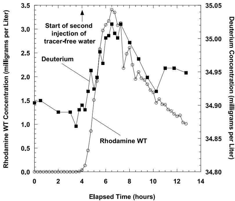
**Figure 6.** Concentration of RWT and  $^2\text{H}$  at production well S-3164 versus elapsed time from the start of tracer injection.
