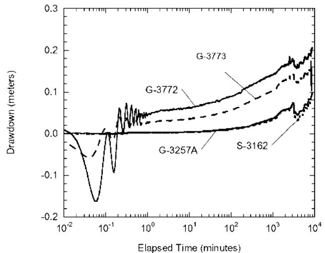
**Figure 5.** Drawdown versus time for selected wells in the NWWF during aquifer test conducted in April 2003.
