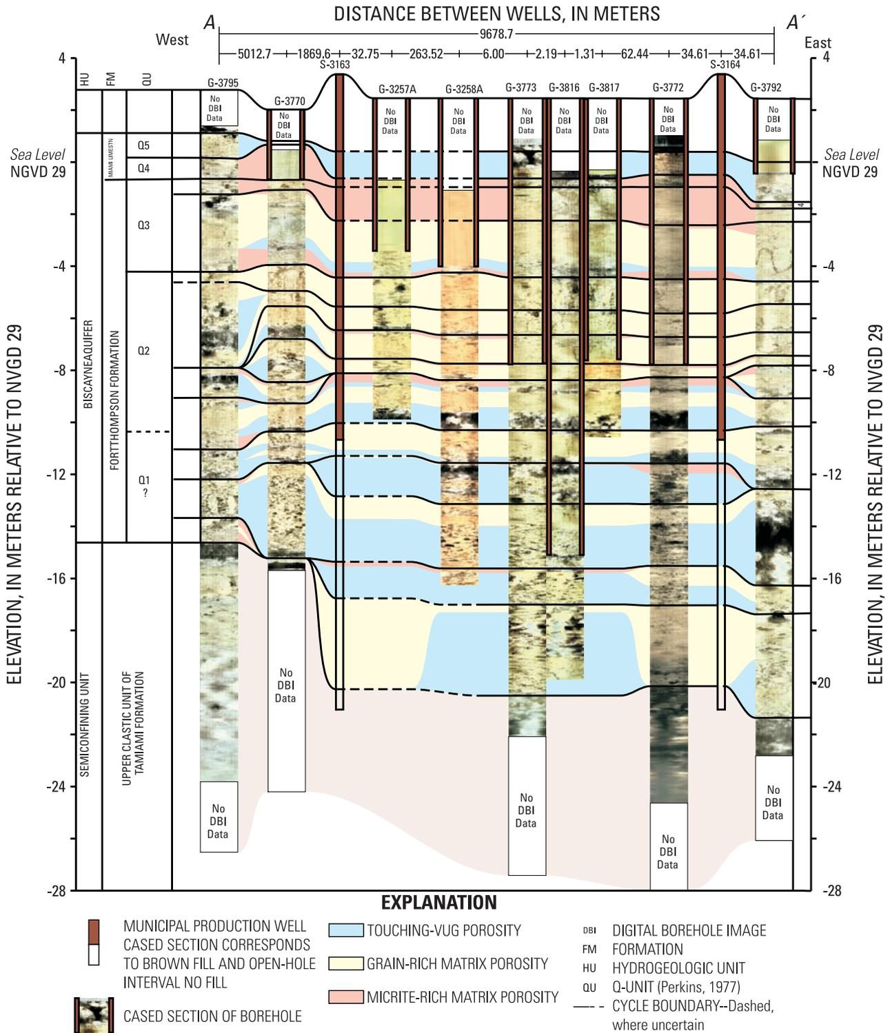
**Figure 4.** Line of section A-A' showing principal geologic and carbonate flow units underlying the NWWF (see Figure 1).
