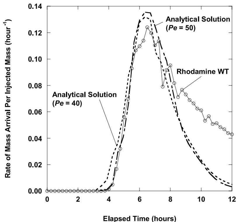
**Figure 10.** Comparison of rate of mass arrival per injected mass versus elapsed time for RWT and analytical solutions for different Peclet numbers for radially converging chemical transport from an injection well to a pumped well.
