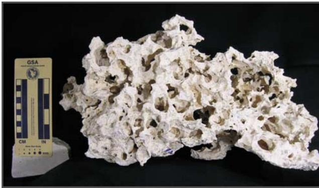
**Figure 3.** Photograph showing touching-vug porosity in a Miami limestone rock sample.
