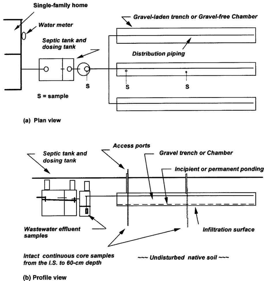
Fig. 2. Illustration of field full-scale system with monitoring locations. IS, infiltrative surface.
