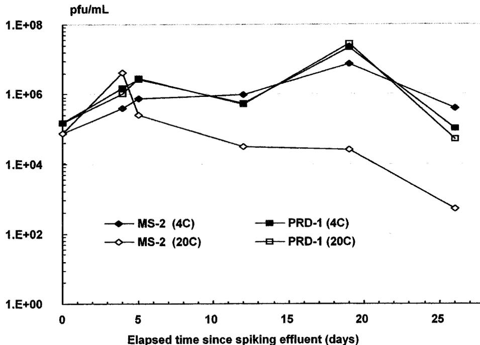
Fig. 8. Bacteriophages MS-2 and PRD-1 in Field Site 2 septic tank effluent (STE) during incubation at 20 and 4°C. Note that all samples were run in duplicate and the average percent difference was 11%.
