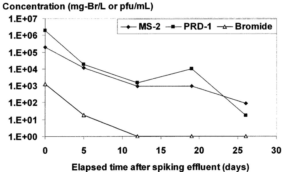
Fig. 6. Concentrations of MS-2 and PRD-1 bacteriophages and the conservative tracer (bromide) in the dosing chamber at Field Site 2 over time.
