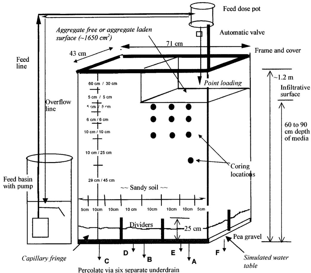
**Fig. 1. Schematic of the three-dimensional pilot-scale soil treatment system.**
