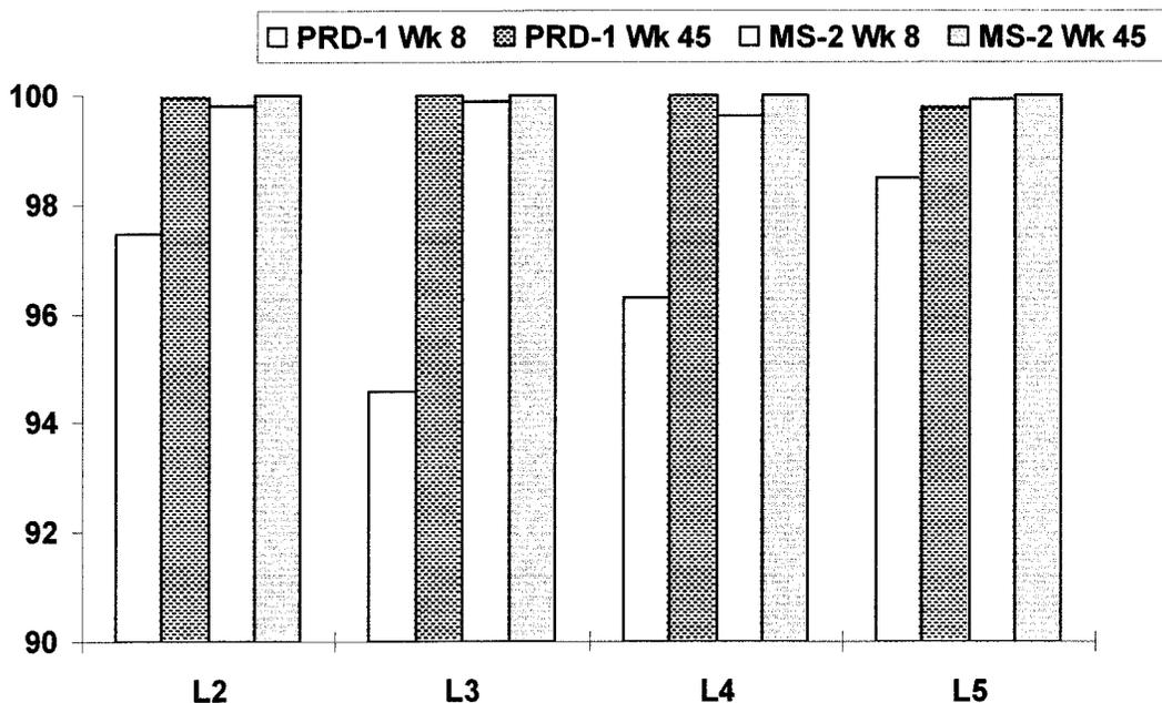
Fig. 4. Percent removal of total applied PRD-1 and MS-2 bacteriophage after 8 and 45 wk of operation. L2, open, 90-cm vadose zone; L3, gravel, 90 cm; L4, gravel, 60 cm; L5 open, 60 cm.
