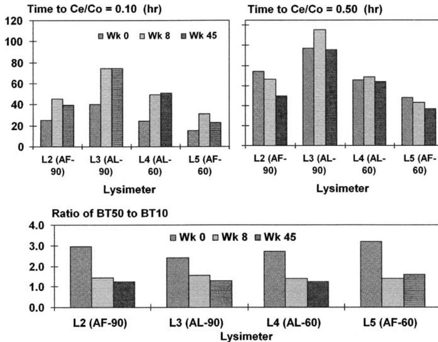
Fig. 3. Time to appearance of bromide tracer in the percolate at 10 and 50% of the applied concentration ( $BT_{10}$  and  $BT_{50}$ , respectively) and their ratio at system start-up after 8 and 45 wk of operation. AF-60, aggregate-free infiltrative surface with 60-cm vadose zone; AL-90, aggregate-laden with 90-cm vadose zone.
