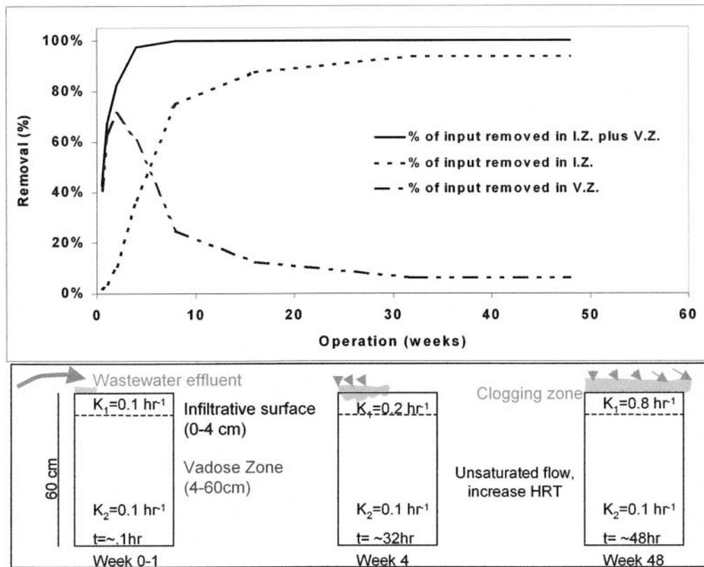
Fig. 11. Virus removal simulation (assuming first-order removal with respect to concentration) with increasing time of operation. Conditions:  $1 \times 10^7$  plaque forming unit (pfu)/mL of virus added in septic tank effluent (STE) dosed at 5 cm/d. IZ, infiltrative zone (0–4 cm); VZ, vadose zone (4–60 cm).
