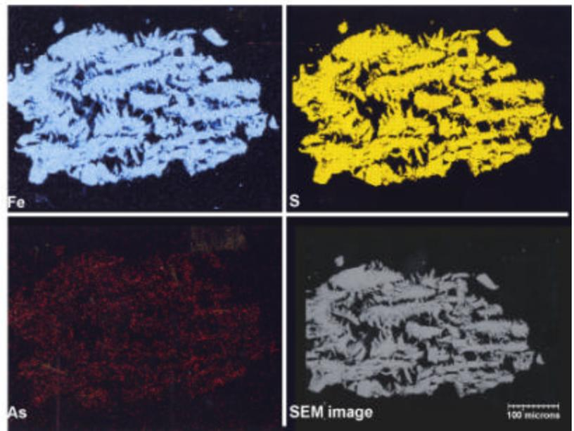
Figure 3. Elemental map of pyrite. Fe=iron, S=sulfur, As=arsenic. SEM= scanning electron microscopy. Scale bar=100
