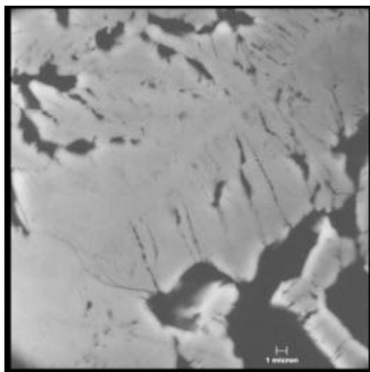
Figure 4. Scanning electron microscopy image of a radiating As-bearing pyrite grain. Scale bar=1 micron.
