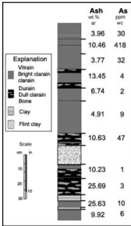
Figure 2. Stratigraphic column of the Fire Clay coal sample.
