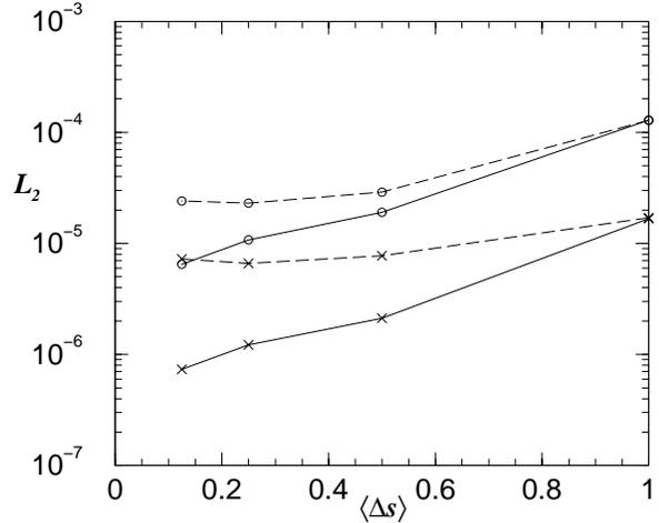
Figure 6.  $L_2$  norm for mesh composed of cells with quasi-random planar faces; see text for  $\langle \Delta s \rangle$ . Solid line: non-linear shape function; Dashed line: linear shape function; Circle:  $d$  is one domain length; Cross:  $d$  is two domain lengths.
