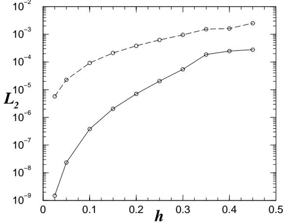
Figure 3.  $L_2$  norm for mesh composed of cells with quasi-random planar faces; see text for  $h$ . Solid line: non-linear shape function; Dashed line: linear shape function.
