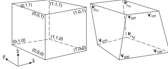
Figure 1. Left: reference cube  $\hat{Q}$  with edges of unit length. Right: arbitrary cell  $Q$  from discretization with vertex locations  $\mathbf{v}_{000}$ ,  $\mathbf{v}_{100}$ ,  $\mathbf{v}_{010}$ ,  $\mathbf{v}_{001}$ ,  $\mathbf{v}_{110}$ ,  $\mathbf{v}_{101}$ ,  $\mathbf{v}_{011}$  and  $\mathbf{v}_{111}$  indicated.
