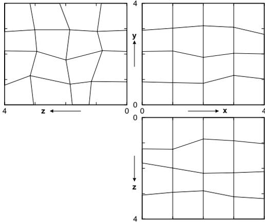
Figure 5. Example of three exterior faces of a  $4 \times 4 \times 4$  domain that share vertex  $(0,0,0)$ . Fold up the left ( $yz$ ) face along the  $y$ -axis and the bottom ( $xz$ ) face along the  $x$ -axis. Randomness of vertex locations is exaggerated.
